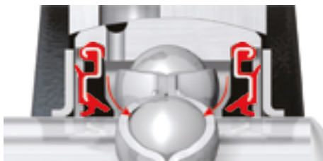
Fig. 3: New seal design for lubrication
