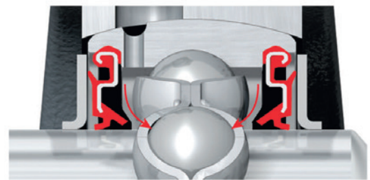
Fig. 3: New seal design for lubrication
