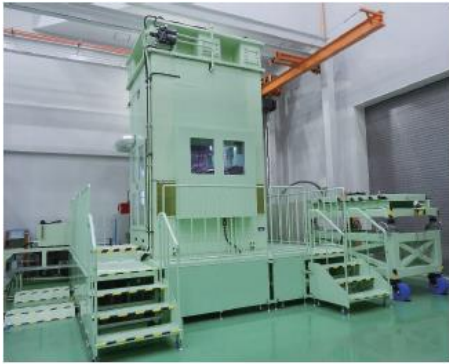
Figure 4: Bearing testing machine for steel production equipment
