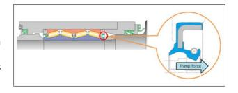
to improve the sealing performance and to significantly reduce the temperature increase and the amount of water intrusion, thereby contributing to a longer bearing service life and a reduction in maintenance costs for our customers.
